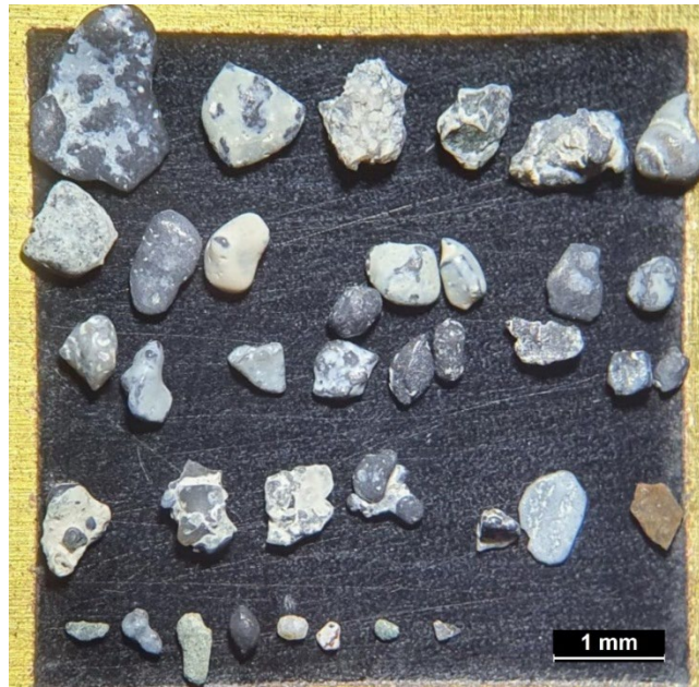
Fig. S 7.28. Binocular microscopy photo with magnifier 10X for 121-123 cm. Variety lithoclasts with different shapes and size are observed in this horizon. The lithoclasts are generally made of Lawsonite, marine cement, aggregate and fossil fractions.
