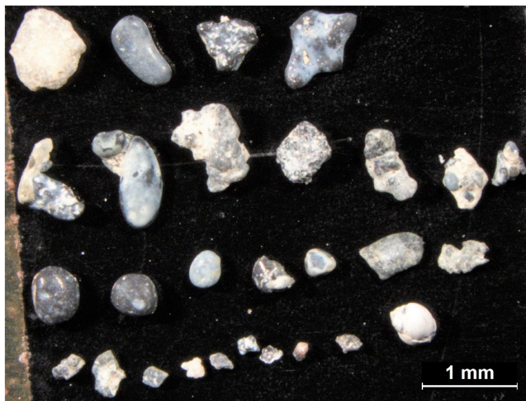
Fig. S 7.4. Binocular microscopy photo with magnifier 10X for 71-73 cm. Variety lithoclasts with different shapes and size are observed in this horizon. The lithoclasts are generally made of Lawsonite, aggregate and fossil fractions.
