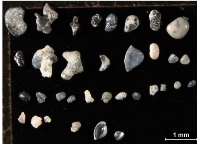
Fig. S 7.19. Binocular microscopy photo with magnifier 10X for 101-103 cm. Variety lithoclasts with different shapes and size are observed in this horizon. The lithoclasts are generally made of Lawsonite, marine cement, aggregate and fossil fractions.
