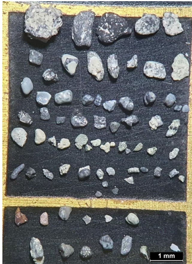
Fig. S 7.21. Binocular microscopy photo with magnifier 10X for 105-107 cm. Variety lithoclasts with different shapes and size are observed in this horizon. The lithoclasts are generally made of Lawsonite, marine cement, aggregate and fossil fractions.
