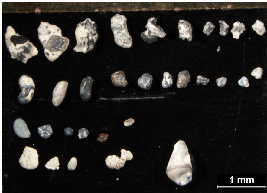
Fig. S 7.14. Binocular microscopy photo with magnifier 10X for 91-93 cm. Variety lithoclasts with different shapes are observed in this horizon. The lithoclasts are generally made of marine cement, aggregate and fossil fractions.
