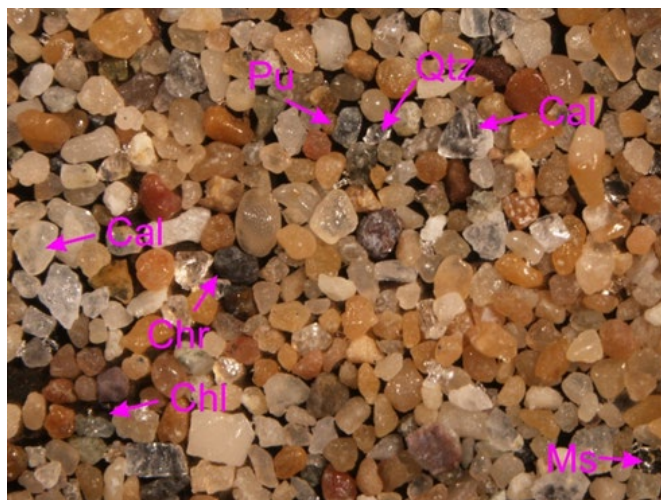
Fig. S 4.10. Binocular microscopy image for Mogham costal sediment with magnifier 11.5X. Cal: Calcite, Ms: Muscovite, Qtz: Quartz, Pu: Pumpellyite, Chl: Chlorite, Chr: Chromite..
