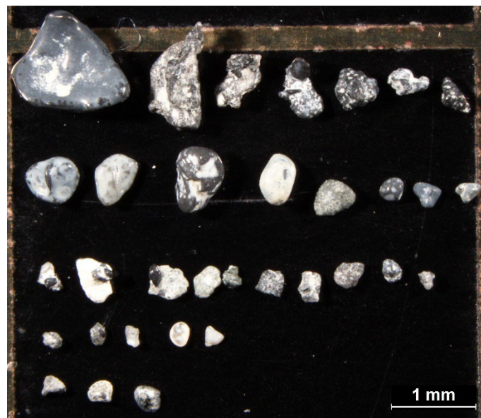
Fig. S 7.16. Binocular microscopy photo with magnifier 10X for 95-97 cm. Variety lithoclasts with different shapes and size are observed in this horizon. The lithoclasts are generally made of Lawsonite, marine cement, aggregate and fossil fractions.
