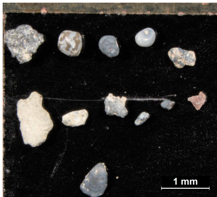
Fig. S 7.2. Binocular microscopy photo with magnifier 10X for 67-69 cm. Variety lithoclasts with different shapes are observed in this horizon. The lithoclasts are generally made of Lawsonite, marine cement, aggregate and fossil fractions.
