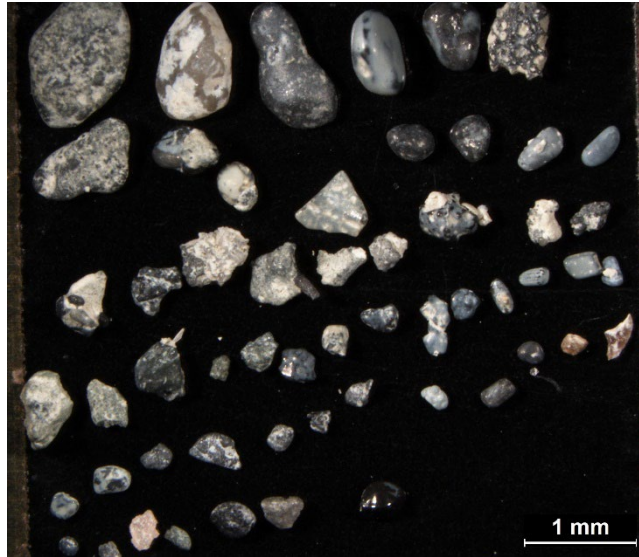
Fig. S 7.13. Binocular microscopy photo with magnifier 10X for 67-69 cm. Variety lithoclasts with different shapes and size are observed in this horizon. The lithoclasts are generally made of Lawsonite, marine cement, aggregate and fossil fractions.
