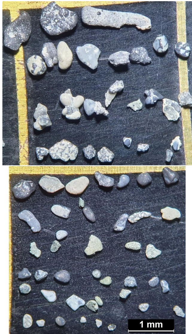
Fig. S 7.27. Binocular microscopy photo with magnifier 10X for 119-121 cm. Variety lithoclasts with different shapes and size are observed in this horizon. The lithoclasts are generally made of Lawsonite, marine cement, aggregate and fossil fractions.
