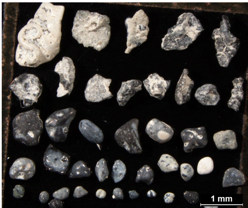
Fig. S 7.18. Binocular microscopy photo with magnifier 10X for 99-101 cm. Variety lithoclasts with different shapes are observed in this horizon. The lithoclasts are generally made of Lawsonite, Glaucophane, marine cement, aggregate and fossil fractions.
