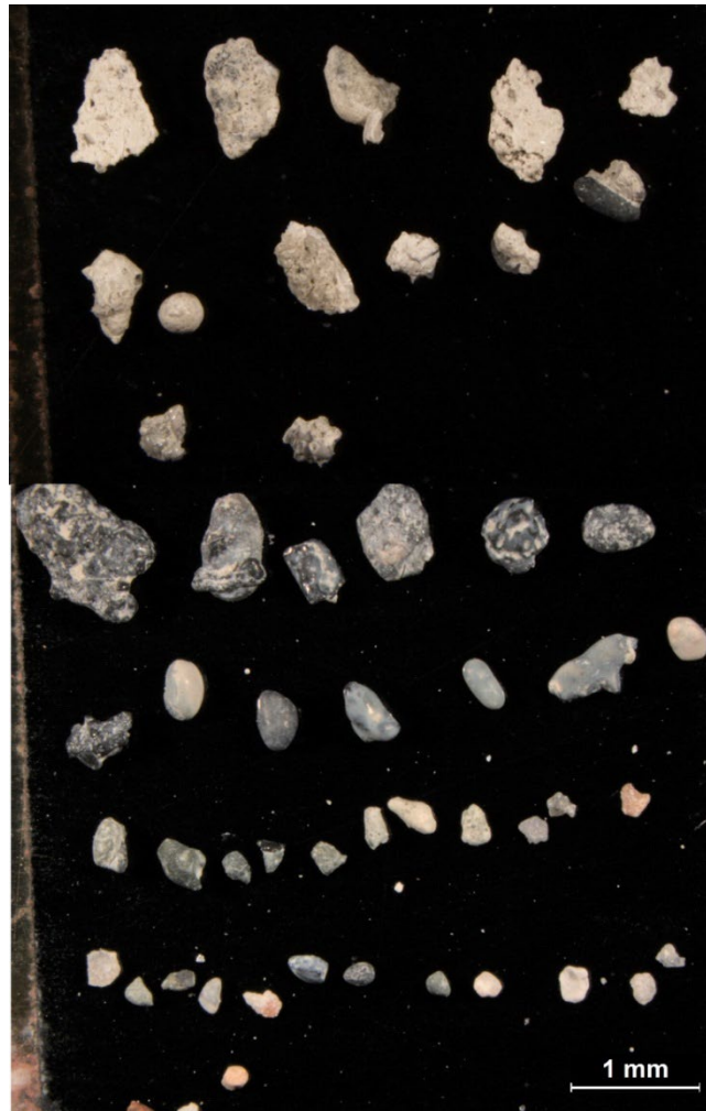
Fig. S 7.24. Binocular microscopy photo with magnifier 10X for 111-113 cm. Variety lithoclasts with different shapes and size are observed in this horizon. The lithoclasts are generally made of Lawsonite, Glaucophane, marine cement, aggregate and fossil fractions.
