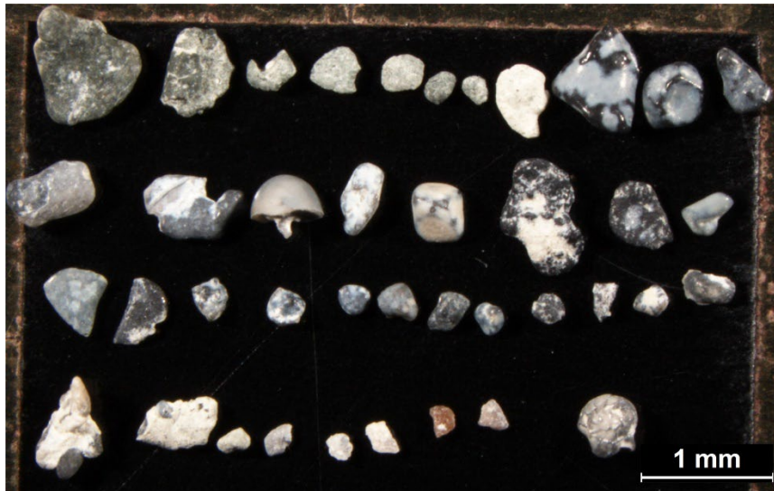
Fig. S 7.15. Binocular microscopy photo with magnifier 10X for 93-95 cm. Variety lithoclasts with different shapes are observed in this horizon. The lithoclasts are generally made of Lawsonite, marine cement, aggregate and fossil fractions.
