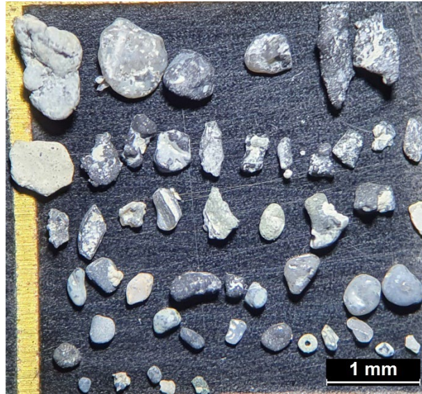
Fig. S 7.30. Binocular microscopy photo with magnifier 10X for 125-127 cm. Variety lithoclasts with different shapes and size are observed in this horizon. The lithoclasts are generally made of Lawsonite, aggregate and fossil fractions.
