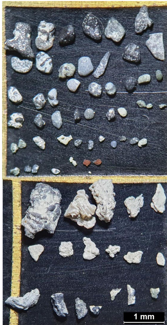
Fig. S 7.25. Binocular microscopy photo with magnifier 10X for 113-115 cm. Variety lithoclasts with different shapes and size are observed in this horizon. The lithoclasts are generally made of Lawsonite, marine cement, aggregate and fossil fractions.
