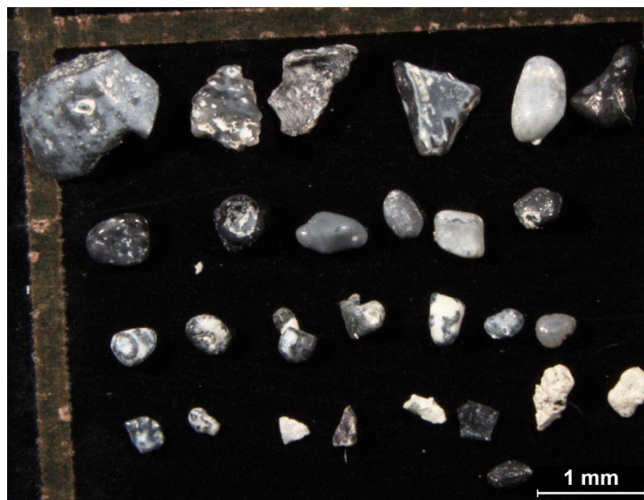
Fig. S 7.6. Binocular microscopy photo with magnifier 10X for 75-55 cm. Variety lithoclasts with different shapes and size are observed in this horizon. The lithoclasts are generally made of Lawsonite, marine cement, aggregate and fossil fractions.
