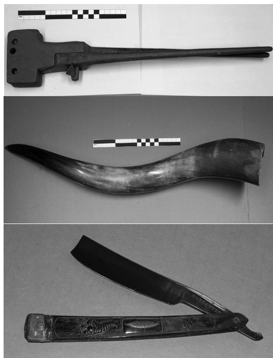
FIG. 6. – Top, horn pressing vice; middle, large cattle horn (courtesy of the Hawley Collection); bottom, 19th century open razor with pressed horn scales. Cutlers' Company collection. Scale in cm.
