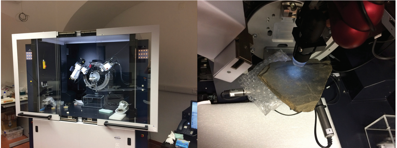
FIG. 6. — X-ray spectroscopy, coupled with scanning electron microscope and by X-ray diffraction.
